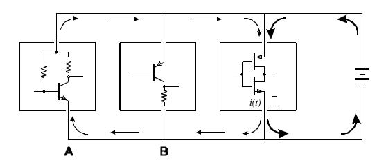
Current also flows into low impedance node A (common base stage), which closes the secondary loop,
