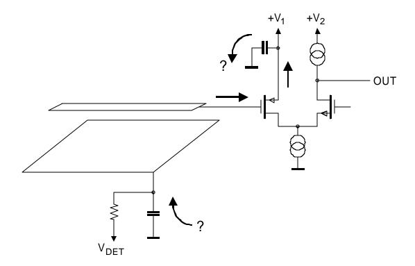
Unless the connection points of the bypass capacitors from the FET source and the detector backplane are chosen carefully, interference will be introduced into the input signal loop.
