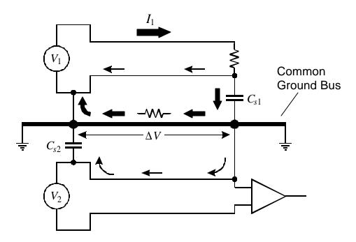
The loops in this figure are the same as shown before, but the loops are closed by the capacitances  $C_{sI}$  and  $C_{s2}$ . Frequently, these capacitances are not formed explicitly by capacitors, but are the stray capacitance formed by a power supply to ground, a detector to its support structure (as represented by  $C_{s2}$ ), etc. For AC signals the inductance of the common current path can increase the impedance substantially beyond the DC resistance, especially at high frequencies.
