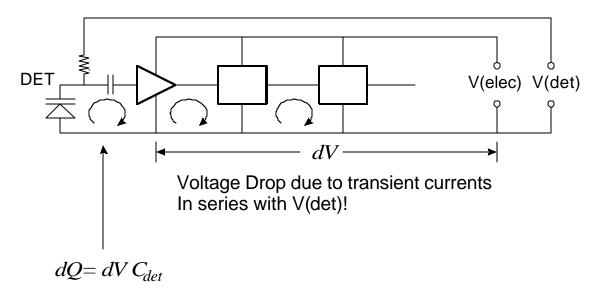
The transient voltage drop dV is superimposed on the detector bias and injects a charge  $dQ = dV C_{det}$  into the input.
