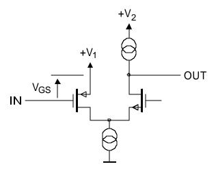
The problem with this configuration is that the supply  $V_1$  becomes part of the input signal path. Unless the  $V_1$  supply bus is very carefully configured and kept free of other signals, interference will be coupled into the input.
