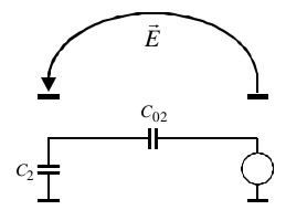
If an intermediate conductor is introduced with a large capacitance to the interference source and to ground compared to the critical node, it will "capture" the field lines and effectively "shield" the critical node.
