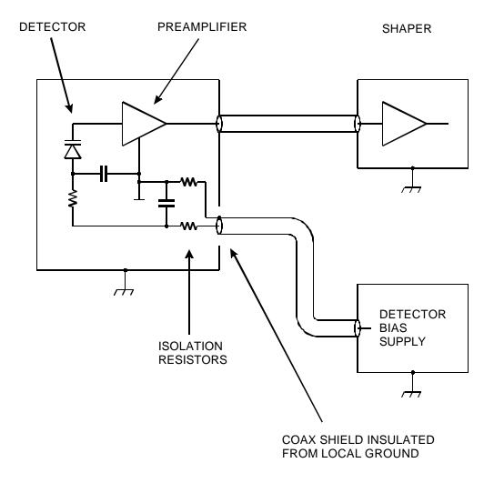
Isolation resistors can also be mounted in an external box that is looped into the bias cable. Either use an insulated box or be sure to isolate the shells of the input and output connectors from another.
