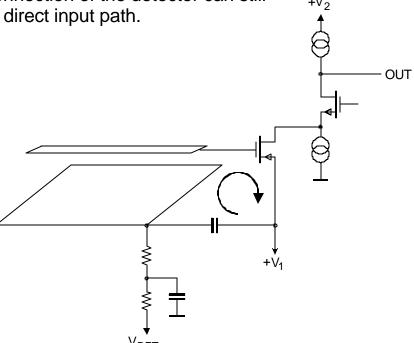
In most implementations supply lines are more susceptible to pickup, so the  $+V_1$  line must be properly filtered to prevent current injection.
