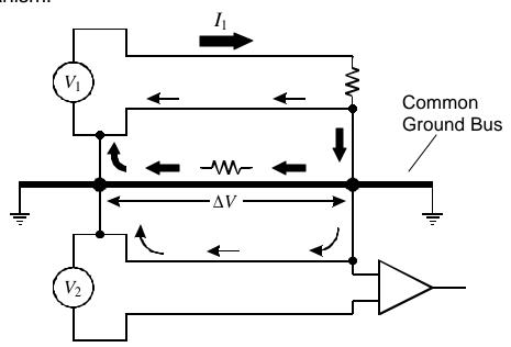
A large alternating current  $I_1$  is coupled into the common ground bus.
