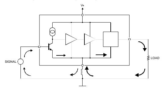
The output current is typically orders of magnitude greater than the input current (due to amplifier gain, load impedance).
