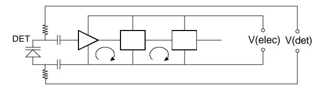
The resistors in both legs of the bias connection isolate the sensitive input node by presenting a high impedance to external signals. Only one of the two capacitors at the input may be necessary, depending on system requirements.
