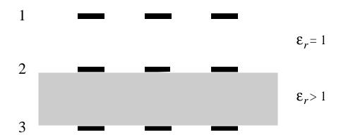
The capacitance between electrode sets 2 and 3 is  $\varepsilon_r$  times larger than between sets 1 and 2.
