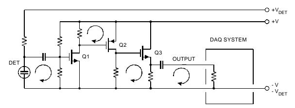
In transferring from stage to stage the signal current flows through local return loops.
