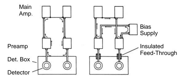
The configuration at the left has a loop that includes the most sensitive part of the system – the detector and preamplifier input.
