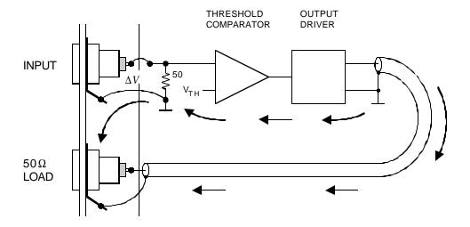
A portion of the output current flowed through the input ground connection. The voltage drop  $\Delta V$  was sufficient to fire the comparator.
