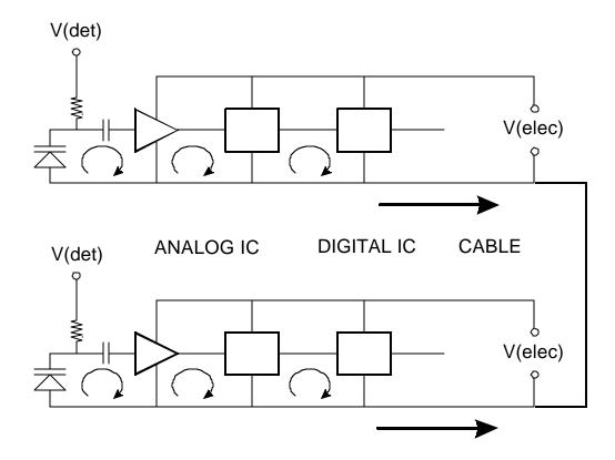
Since the path of least resistance is provided by the cabling and connections to the power supplies and data acquisition system, current transients originating in the front-end circuitry do not flow towards the input.
