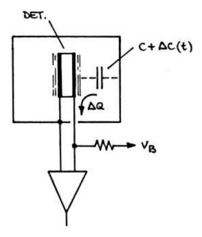
If the electrode at potential  $V_B$  vibrates with respect to the enclosure, the stray capacitance C is modulated by  $\Delta C(t)$ , inducing a charge
