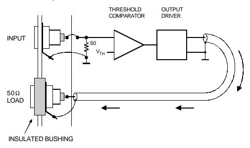
Often it is convenient to replace the coax cable at the output by a strip line integrated on the PC board.
