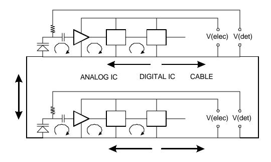
Since the cross-connection at the input is formed by the connection of multiple chips to the detector, it is unavoidable.
