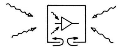
External fields can penetrate significantly if openings > 1/1000 (diameter of holes, length of slots).
